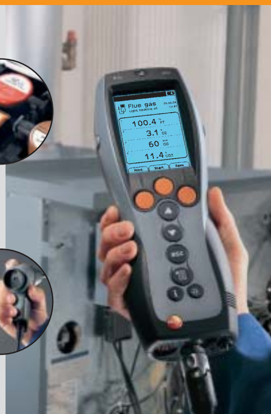
Flue gas analysis on oil and gas heating systems
