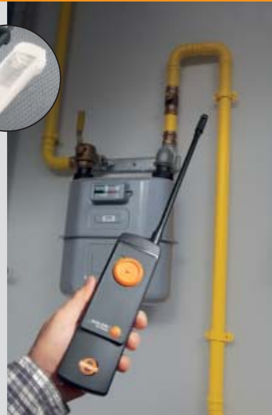
Checks for leaks in domestic gas pipes
