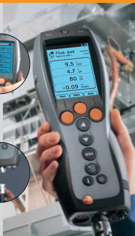
Flue gas analysis on atmospheric gas burner systems
