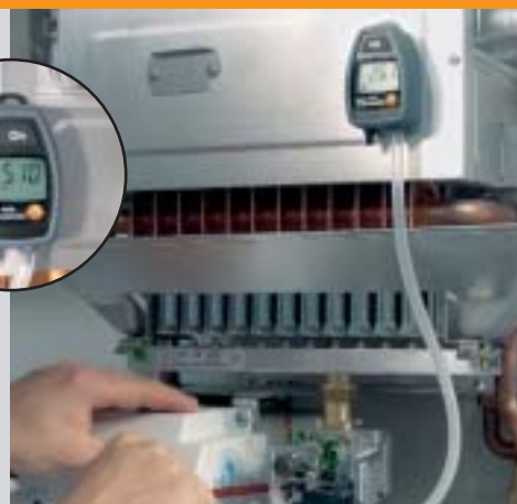
Switchable measurement range; gas flow pressure and flue draught measurement
