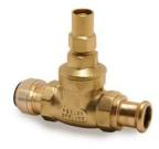
Brass full way gate valve with lockshield. XPress press end x Tectite push end for copper/carbon steel/stainless steel tube.
