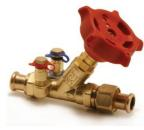
Commissioning Valve (FODRV).DZR brass body with test points. Xpress union outlet x Xpress end for copper, carbon/ stainless steel.
