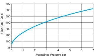
The pressure loss/flow rate graphs are for the controller only at midblend and do not take account of pressure loss through check valves, in-line fittings, pipework or terminal fittings. When calculating the pump rate for the circuit allow 0.01bar for pressure loss through the Rada 32rmx at 10 l/min.
