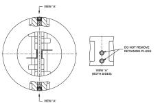
**NOTE:** The valve must be installed with the direction arrow on the body coincident with the direction of flow in the pipeline. For vertical pipework the flow direction should be upwards only.
