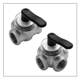
Danfoss HRB rotary valves are primarily designed for regulation of flow temperature in heating systems where a certain leakage can be accepted and where a defined control characteristic is not required. HRB rotary valves can be used in combination with electric actuators AMB 162 and AMB 182.
