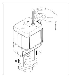
The manual override is applied by rotating the 4 mm Allen key (not supplied) to the required position. Observe the direction of the rotation symbol.
