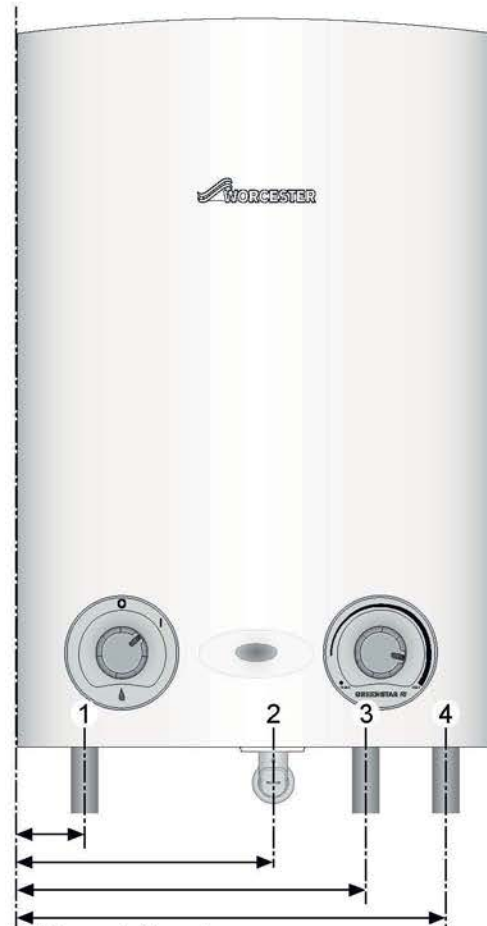
Fig. 19 Pipe work dimensions
