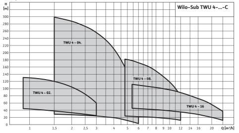
1~230 V or 3~400 V, 50 Hz, p = 1 kg/dm3, v = 1x10-6 m2/s, ISO 9906 Annex A,  $\eta$  = pump efficiency
