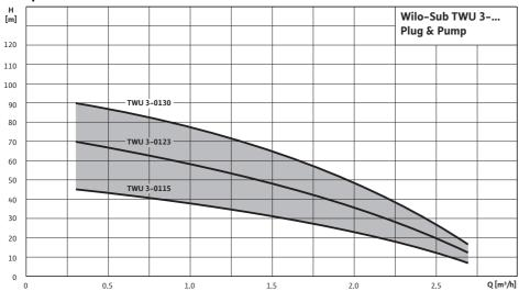
$1\sim230$  V, 50 Hz, p=1 kg/dm3, v=1x10-6 m2/s, ISO 9906 Annex A,  $\eta=$  pump efficiency
