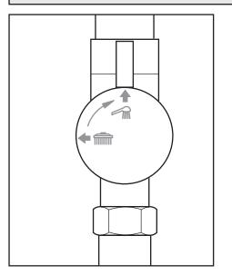
To divert the water from the handset to the riser, turn anti-clockwise.
