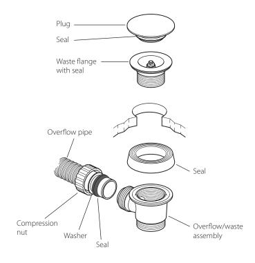
Push the seal onto the waste assembly
