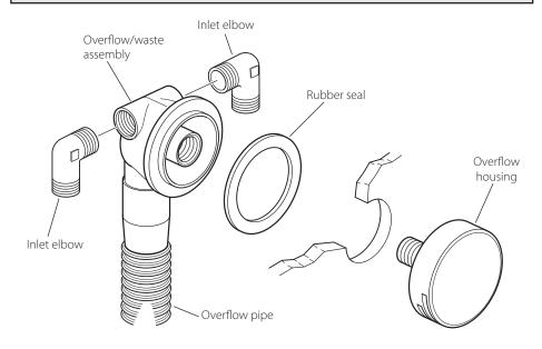
Remove the blanking plug from the overflow assembly. Using PTFE tape fit the two inlet elbows.
