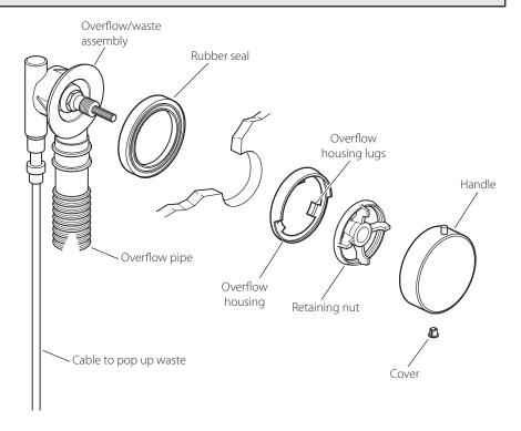
Push the rubber seal onto the overflow/waste assembly, and from the outside push the shaft through the bath overflow hole and hold in place.
