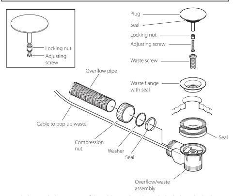
From below push the top part of the rubber seal up through the hole in the bath. Push the waste housing up into the seal and hold in place.
