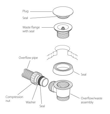
Push the rubber seal onto the overflow/waste assembly, screw in the shaft and from the outside push through the bath overflow hole, hold in place.
