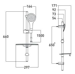
\* The riser rail wall brackets can be positioned as required. This allows any existing holes to be re-used or covered by the wall brackets. The brackets can also be adjusted to sit in the middle of tiles or within the tile joints.
