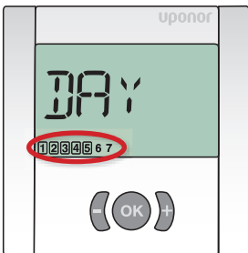
12. Select schedule group. Press + or - successively to select the group of days. There are three alternatives: • 1 2 3 4 5 6 7 Monday till Friday, default setting. • 1 2 3 4 5 6 7 Monday till Saturday. • 1 2 3 4 5 6 7 Monday till Sunday.
