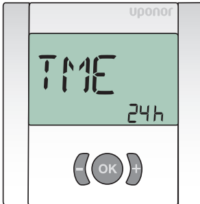
7. Choose between 24hr or 12hr time clock, confirm by pressing OK.
