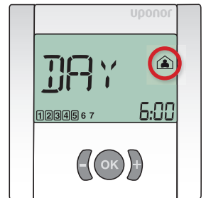
15. Example shows 6am as the chosen comfort event. Press OK to put the person in the house.
