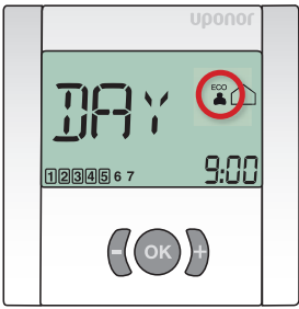
16. Example shows 9am as the next chosen ECO event. Press OK to take the person outside of the house.
