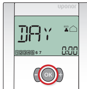
13. To accept the default setting press and hold the OK button for 3 seconds. Repeat for Z2 and subsequent group day(s) if applicable.
