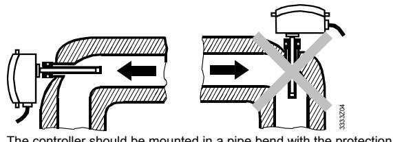
The controller should be mounted in a pipe bend with the protection pocket facing the flow.
