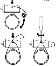
Building Technologies HVAC Products Clamp-on temperature sensor QAD2...
