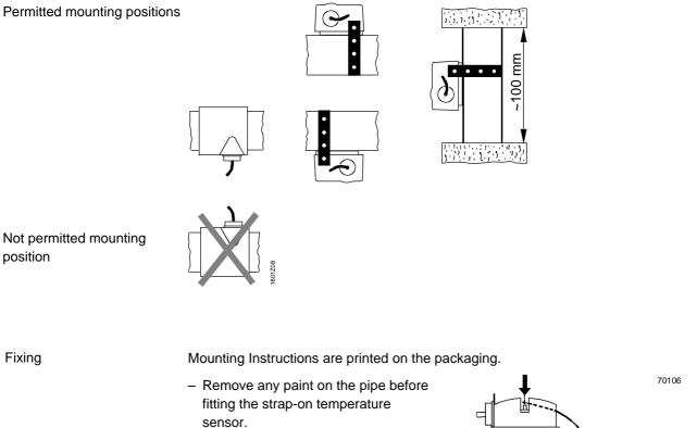
Ensure that the sensor is fixed firmly with the adjustable band supplied.
