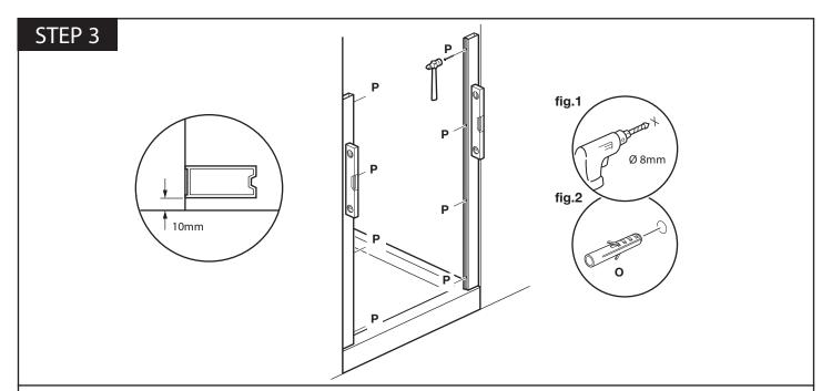
Position the wall channels 10mm from front edge of the tray using the measuring tool (W). Holding the wall channels to the wall and ensuring they are perfectly vertical and parallel to each other, mark off drill hole positions onto the tiles using centre punch (P).
