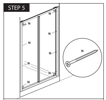
Lift and place the enclosure onto the tray, seek assistance should you require it. The enclosure should sit with an even gap all along the front of the tray with no part overhanging. Line up the enclosure with the pre drilled holes in the walls. Using the 65mm countersunk screws (**N**) fix through the enclosure sides into the fitted wall plugs.
