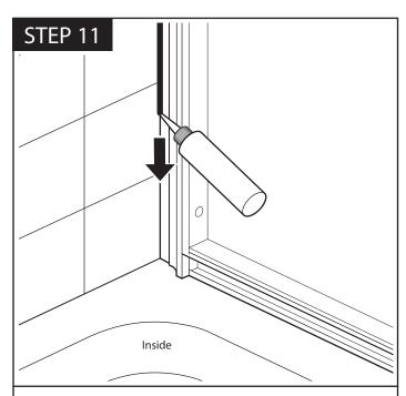
From the inside of the shower enclosure, silicone the entire vertical length of the wall channels up against the walls.
