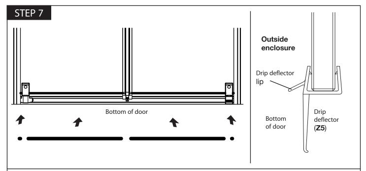
Take one of the drip deflectors (Z5) and size a short piece from it to fit between the frame and the pivot block, trim this sized piece from the drip deflector and fit. Repeat this with the other drip deflector (Z5) between the frame and the wheel hanger.
