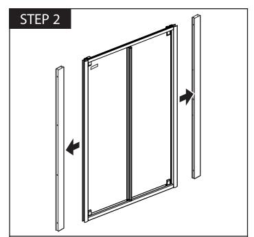
Remove the wall channels from the door and put to one side.
