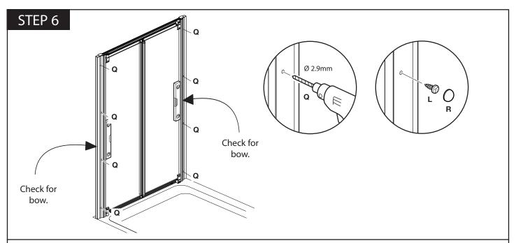
With the tray level, centre the enclosure within the wall channels and ensure the frame is vertical.
