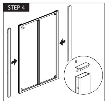
Fit the wall channel caps (**S**) to the top of the wall channels with the end tab (\*) in the position shown. **Note:** Tapping in place with a rubber mallet may help.
