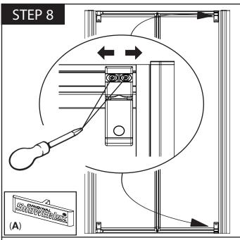
It is important that the door is kept square within the frame to allow the door to run freely.
