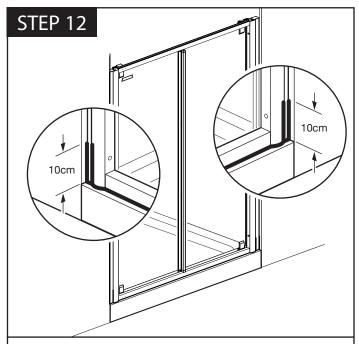
From outside the enclosure, silicone along the bottom of the enclosure on the shower tray all the way around and 10cm up each wall.
