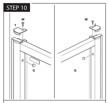
Place the correctly handed frame caps ( $\mathbf{T} \& \mathbf{J}$ ) as shown and fix using 13mm countersunk screws ( $\mathbf{M}$ ).
