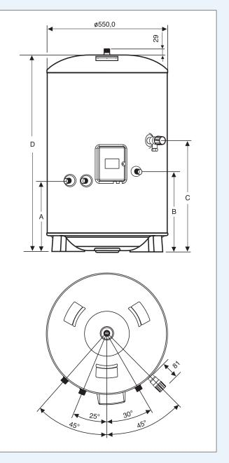
Note A. A third element boss is supplied blanked off to enable an additional 3kW @ 240V element to be fitted if required. For additional element, order Code No. 94 970 036
