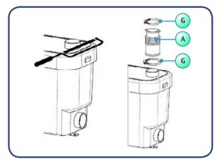
To connect to a lid inlet, cut off the sealed cap with a hacksaw and connect using the rubber connector (A) provided. Tighter with the metal hose clips (G).
