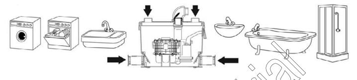
This unit is a pump that will clear the waste from a domestic shower and washbasin, bath, washing machine, glass washer and a sink.
