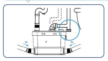
For possible service requirements, provide a drain off at the low point of the installation.
