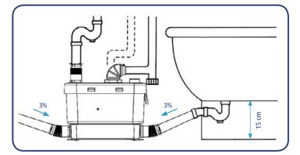
To connect a shower/bath, ensure that the trap exit is 15cm above floor level. Although not obligatory, a lid connection may be used to run an external air vent.
