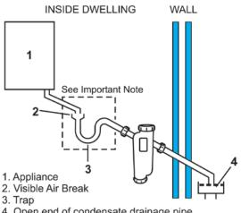
Open end of condensate drainage pipe direct into gully below grating but above water level
