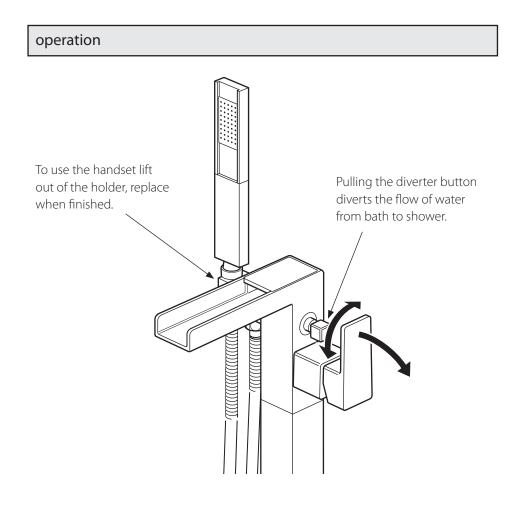
Pull the control lever out to increase the flow of water. Moving the control lever anti-clockwise will decrease the water temperature.
