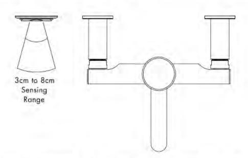
As the sensor is activated the delivery of water will commence, the mixer is factory set to deliver water at a pre-set maximum temperature of 43°C.
