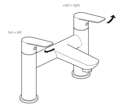
Moving the levers in the direction of the arrows will increase the flow of water.
