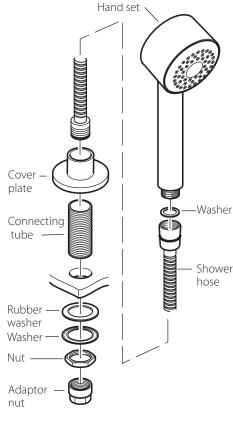
Screw the connecting tube into the cover plate and position in the hole, from the underside slide on the rubber washer, metal washer and then the nut. Tighten the nut to clamp on the spout.
