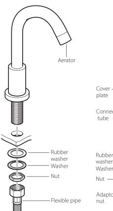
Position the spout in place, and from the underside slide on the rubber washer, metal washer and then the nut. Tighten the nut to clamp on the spout.
