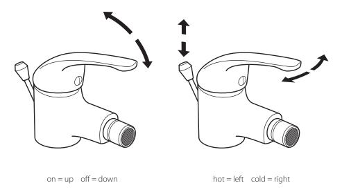
Moving the mixer lever upwards/downwards will increase/decrease the flow of water.
