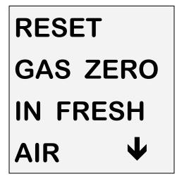
This message indicates that the analyser needs to be reset in fresh air. To do so, ensure that the analyser is in fresh air and press Send / S
