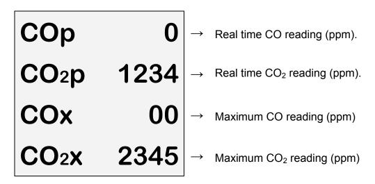
These reading can be printed by quickly pressing the PRINT/SEND key or can be stored in memory by pressing the PRINT/SEND key until the analyser beeps and a log number appears on the top line of the display
