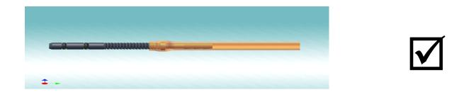
Push 'orange' tube over the rim of the spigot to ensure a gas tight seal.
