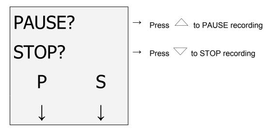
If PAUSE is selected the display will change to 'Paused Screen'. In paused mode the 'live' CO readings are displayed but not recorded.
