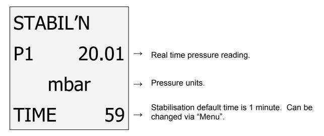
When complete readjust the gas pressure if necessary then press to start the tightness test:
