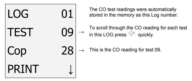
When completed the log can be printed immediately by pressing 2 seconds.
