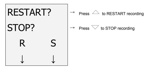
If RESTART is selected the display recerts to the 'Measure and Record Screen'. CO readings are displayed and recorded at the interval originally selected.
