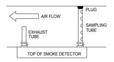
Fit the sampling tube across the entire width of the duct.
