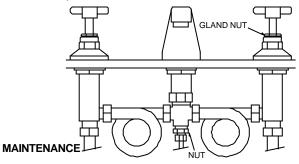
Traditional valve type: - If the fitting leaks from the spindle
