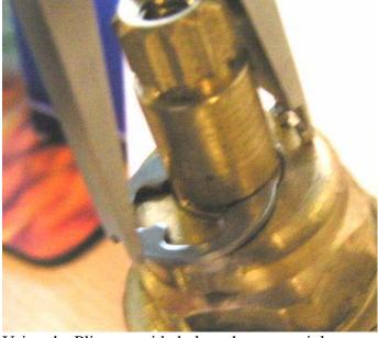
Using the Pliers provided place the new stainless steel 'E' clip (Provided) steadying the clip with one hand.
