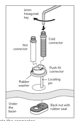
Important: The push-fit connector must be fully tightened to the back nut before attaching the flexible connecting pipes.
