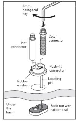
**Note**: The hot connector has 2 flat edges at the top to allow it to fit fully down and close to the top of the cold
