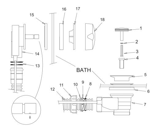
PLEASE NOTE: DO NOT PUSH THE HANDLE (18) ONTO THE SPINDLE (RINGED) OF THE OVERFLOW ELBOW (14), AS THIS WILL STOP WATER COMING OUT OF THE OVERFLOW.
