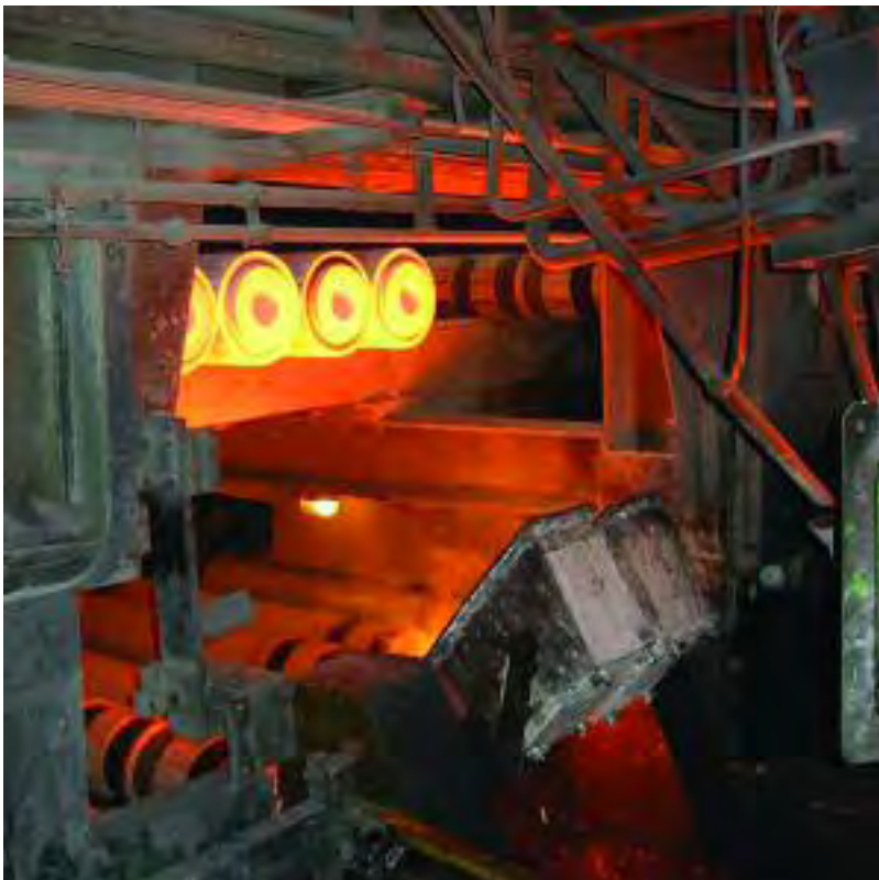
Centrifugal casting process
