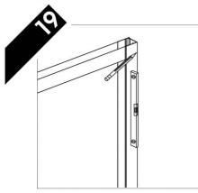
Make sure both wall profiles are upright using a spirit level. Mark the wall along the length of the profiles. Remove the assembly from the tray.
