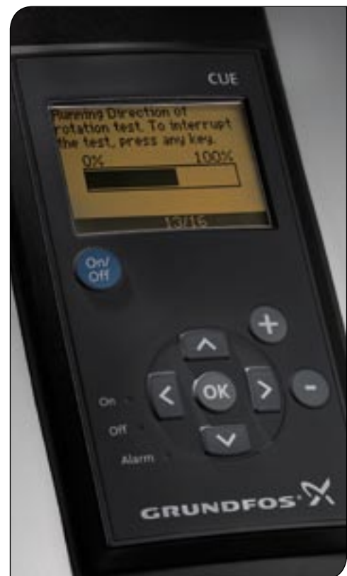
Automatic detection and setting of correct direction of rotation
