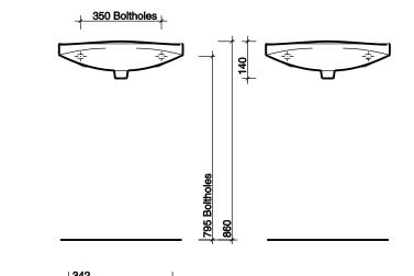
All measurements shown are in millimetres. Drawing sizes
