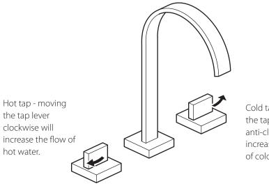
Cold tap - moving the tap lever anti-clockwise will increase the flow of cold water.
