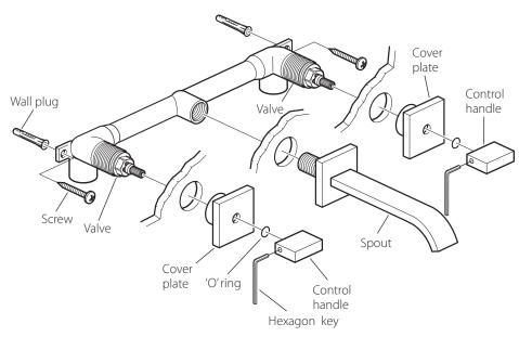
Before installing your new mixer, flush through the pipework to ensure removal of debris, turn off the water supply.
