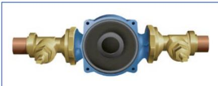
3. Connect your power flushing pump to the PPHA. Use only PLASTIC (PP) 3/4" female nut liner and seals, as provided with the Fernox Powerflow pump and PPHA. Secure these to the hoses with screw clamps. The use of metal connectors will damage the thread on the PPHA fittings and reduce its service life. Note that the kidney shaped port on the PPHA is the flow to the system (F); whilst the central port with the sprung sliding bush is the system return (R).
