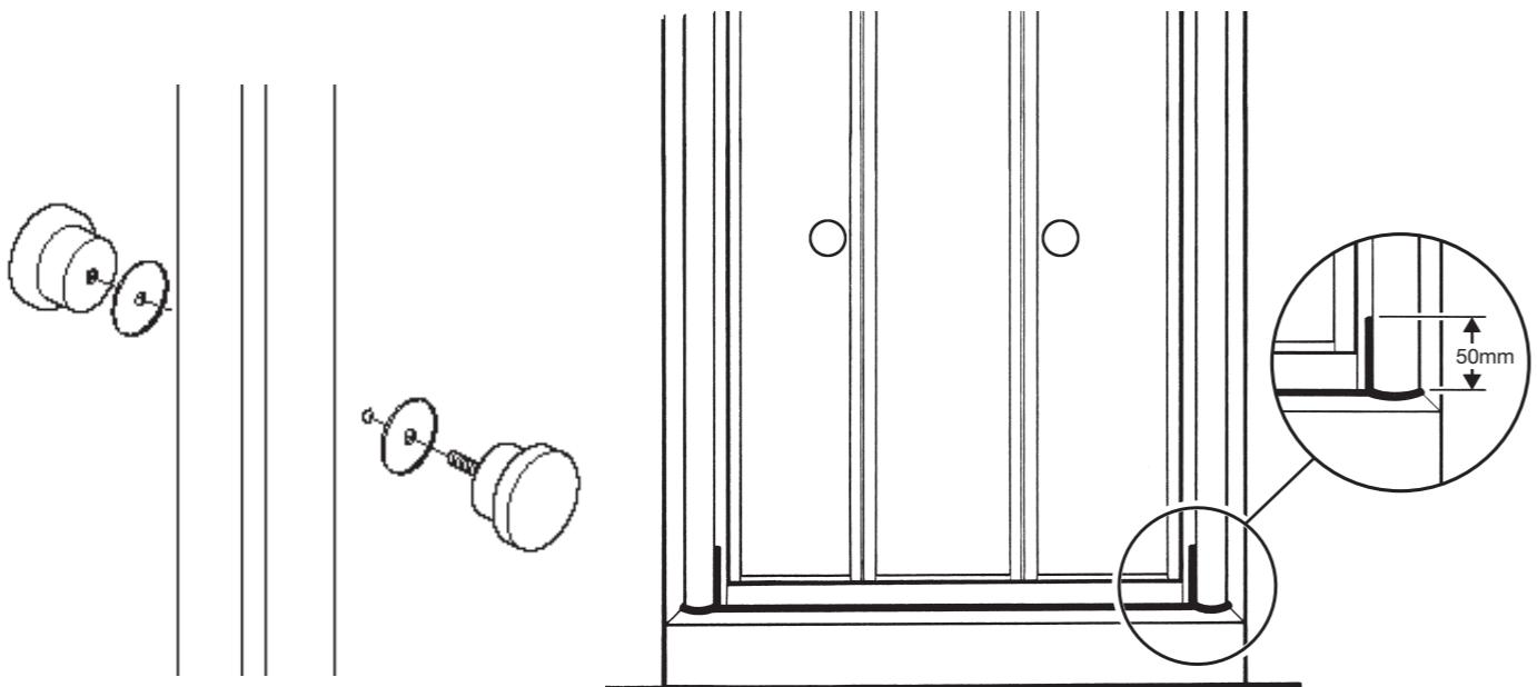
**GB** Fit door handles to the door ensuring the supplied handle washers are used on each side of the glass. (A chrome finish handle is supplied with all frame finish options)
