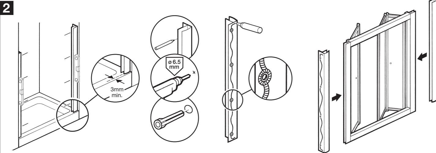
**GB** Place wall channels on tray ensuring they are vertical and a minimum of 3mm back from the front of the tray. Place masking tape against the wall before marking drill hole positions. This will help prevent the drill bit slipping. Drill 6.5mm holes, 30mm deep and insert wall plugs. Apply sealant to the back of wall channels. Place wall channels onto door.
