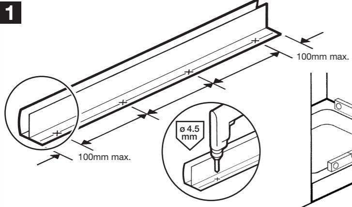
**GB** Drill holes in both wall channels at points shown using a 4.5mm drill bit, through the edge shown and between the grooves. Ensure shower tray is level in all directions.
