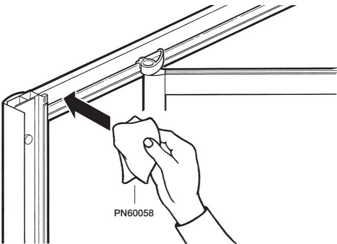
**GB** Move doors and lubricate top and bottom door runners with wipe provided.
