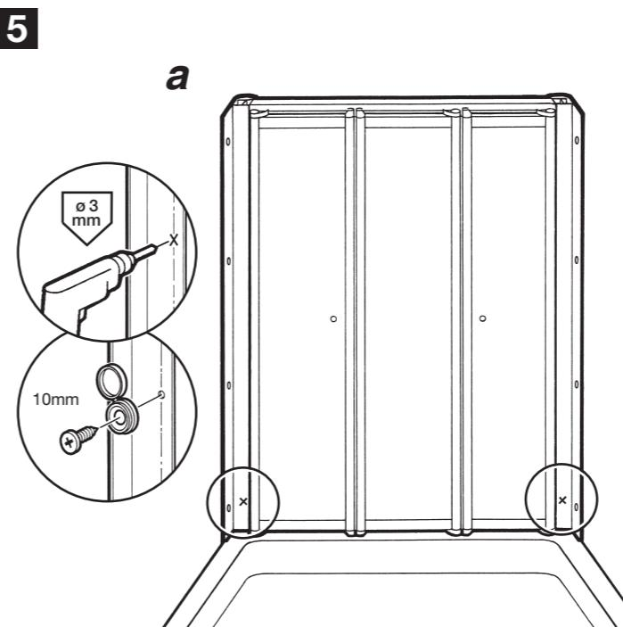
**GB** Check door is centrally positioned and perfectly vertical. Drill inside of wall channels using 3mm drill bit in the two lower positions. Fix using 10mm screws (a).
