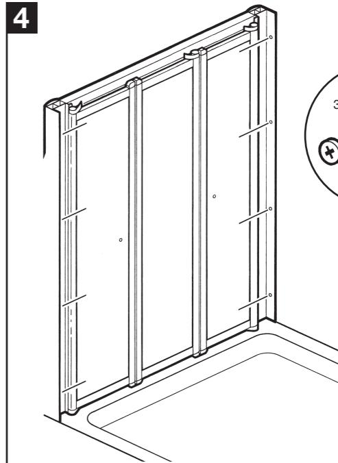
**GB** Place door in position on the tray, fix wall channels to walls using 32mm screws.
