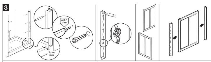
Place wall channels on the tray ensuring they are vertical and a minimum of 3mm back from the front of the tray. Place masking tape against the wall before marking the drill hole positions (this will prevent the drill bit slipping). Drill 6.5mm holes, 30mm deep and insert wall plugs.
