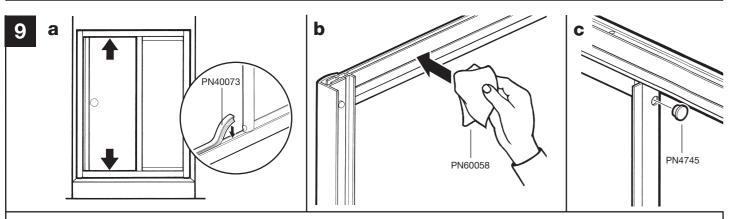
(a) Push-fit the threshold strip (PN40073) in to top and bottom rails. Cut to length, ensuring they fit right up to the end of each rail. (b) Lubricate inner top and bottom rails with wipe provided. (c) Push fit the two hole plugs (PN4745) at the top and bottom of the fixed panel
