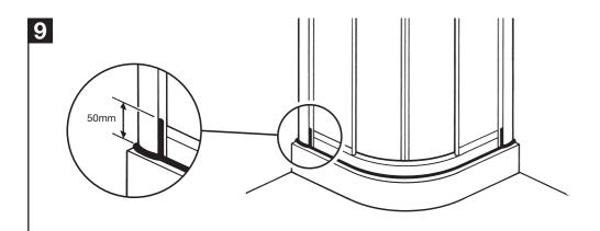
From the outside only, apply sealant to the bottom of the enclosure and 50mm up the wall channels as shown.
