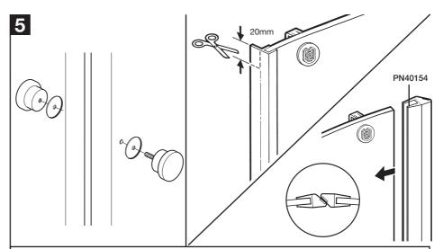
Fit door handles ensuring the supplied handle washers are used on each side of the glass (A chrome finish handle is supplied with all frame finish options. **DO NOT OVER TIGHTEN**, finger tighten only.
