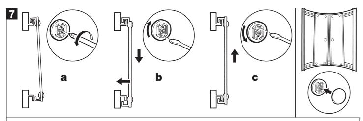
(a) Loosen top hanger screws (1 turn maximum) on doors. (b) Rotate top mouldings until bottom mouldings hook under bottom rail. (c) Rotate top mouldings to lift doors back up (with bottom sliders hooked under rail), re-tighten hanger screws. Doors may need adjusting (as in a, b & c) so they are square, meet in the middle and slide freely.
