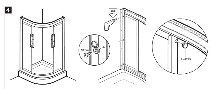
Slot enclosure into the wall channels, one side at a time. Two people may be required for this procedure. Check enclosure is vertical. Drill inside of wall channels using 3mm drill bit where shown. Do not drill too deep. Fix using 10mm screws and screw caps. Push fit all 4 hole plugs top and bottom of fixed panels.
