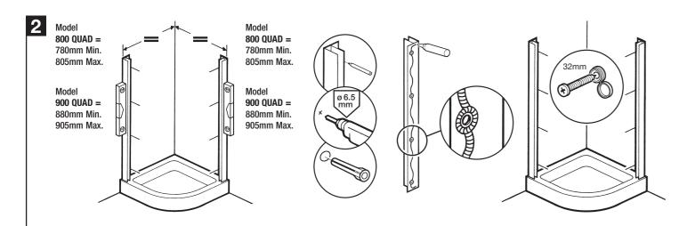
Place wall channels on tray as shown (to fit within the dimensions above), ensuring they are vertical. Place masking tape against the wall before marking the drill hole positions. This will prevent the drill bit slipping. Drill 6.5mm holes – 30mm deep, insert wall plugs and apply sealant to back of wall channels. Fix to walls using 32mm screws and screw caps.
