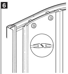
Hang doors on to top track of the frame. Ensure the seal meet as shown.
