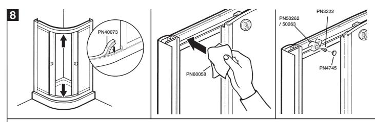
Push fit threshold strip to top and bottom rails. Cut to length, ensuring they fit up to each fixed panel. Lubricate inner top and bottom rails with wipe provided. Fit doorstops using 10mm screws and push fit screw cover cap (PN4745).
