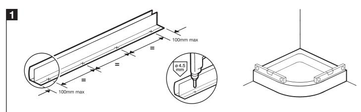
Drill holes in both wall channels (PN10453) at points shown using a 4.5mm drill bit, through the edge shown and in the grooves. Ensure shower tray is level in all directions.
