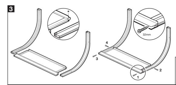
Screw fixed panels to the rails using 32mm screws
