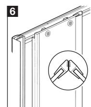
Hang the doors on to top track of the frame. Ensure the seals meet as shown.
