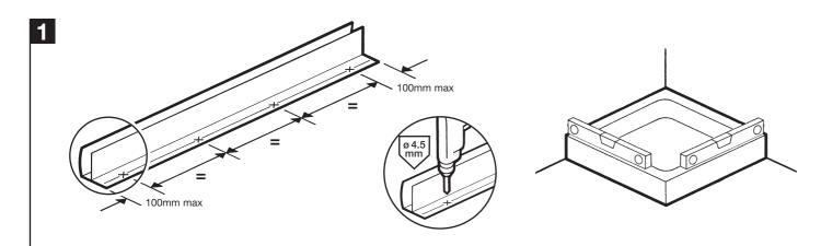
Drill holes in both wall channels (PN10453) at points shown using a 4.5mm drill bit, through the edge shown and in the grooves. Ensure shower tray is level in all directions.
