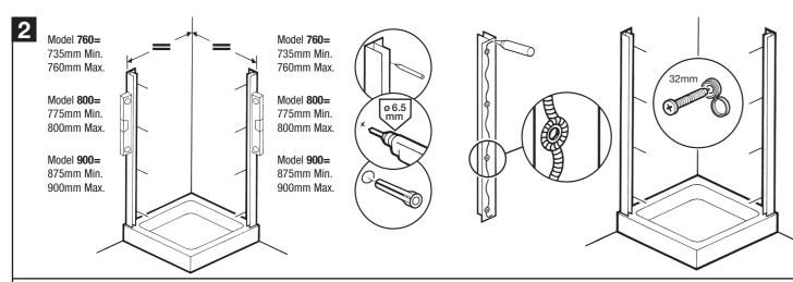
Place wall channels on tray as shown (to fit within the dimensions above), ensure they are vertical. Place masking tape against the wall before marking the drill hole positions, this will prevent the drill bit slipping.
