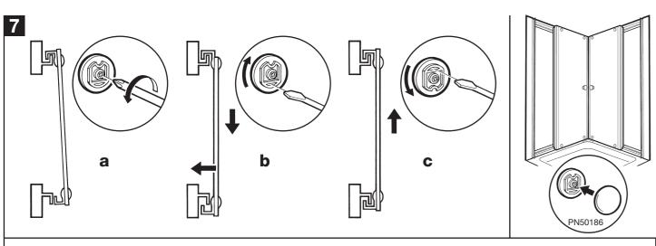
Doors may need adjusting (as in a, b & c) so they are square, meet in the middle and slide freely. (a) Loosen top hanger screws (1 turn maximum) on doors. (b) Rotate top mouldings until bottom mouldings hook under bottom rail. (c) Rotate top mouldings to lift doors back up (with bottom sliders hooked under rail), re-tighten hanger screws.
