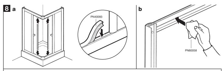
(a) Push-fit threshold strip (PN40093) in to top and bottom rails. Cut to length, ensuring they fit up to corner mouldings.
