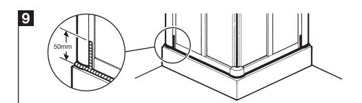
From the outside only, apply sealant to the bottom of the enclosure and 50mm up the wall channels as shown.
