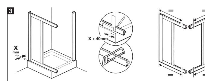
Insert a side panel into a wall channel. If required mark and cut the bottom rail as shown. Measure the cut rail and cut the remaining top and bottom rails to the same length.
