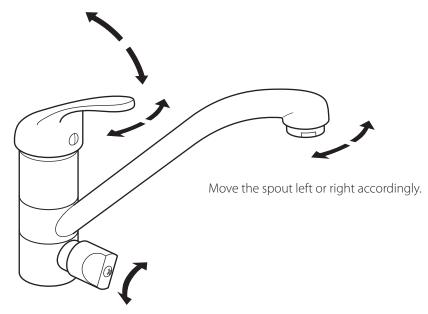
With the mixer lever in the OFF position, turn the handle anti-clockwise to increase the flow of filtered water. Turn clockwise to decrease the flow of water from in-line filter (not supplied).
