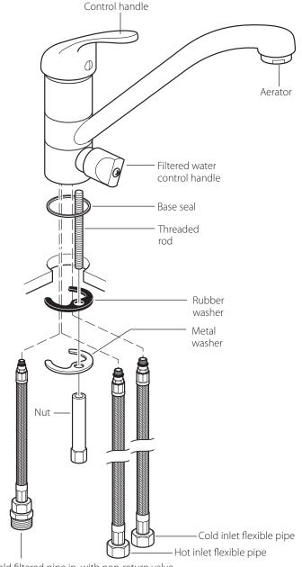
Cold filtered pipe in, with non-return valve
