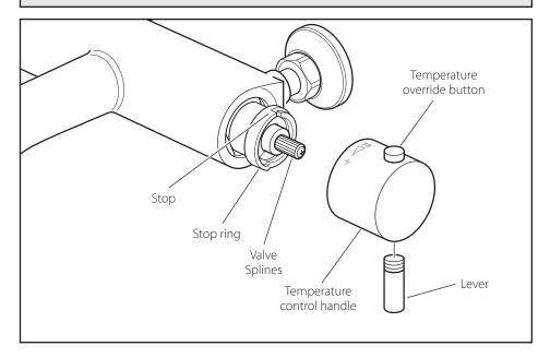
The valve has been factory set under balance pressures and hot water supply at 65° C. When your specific operating conditions are significantly different from the above, the temperature of the water may vary from the setting.
