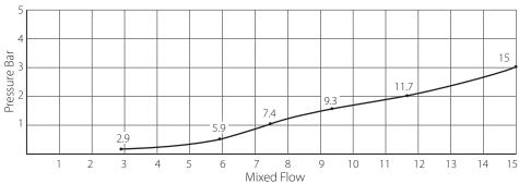
Flow rate curve is for reference only. The actual pressure drop may vary depending on system temperature and pressure.
